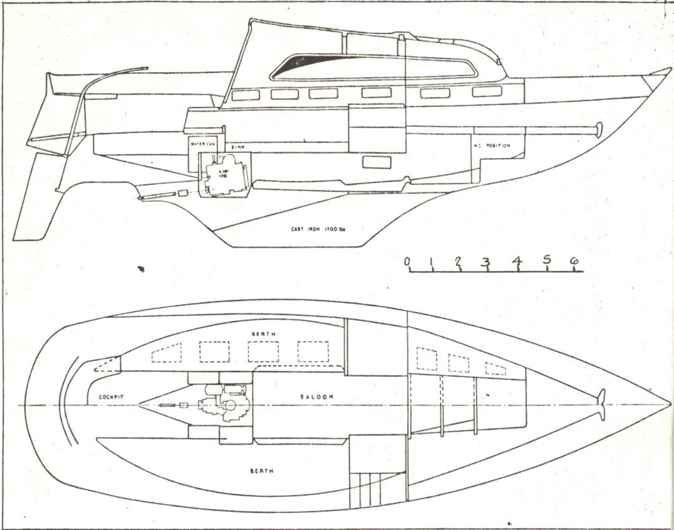
(above) The accommodation is light and airy and laid out on an open plan. There is useful headroom of 5ft 9in beneath the coachroof.
