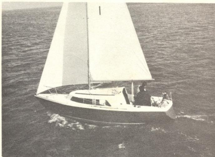
GALION comes ready to sail, with alloy spars, jib and mainsail in Terylene, stainless steel rigging; sheets and halyards; anchor, chain and warps.
