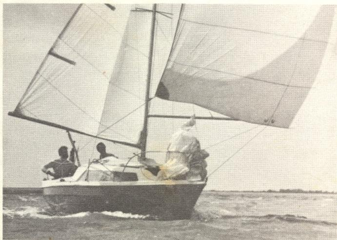
Reinforced glass fibre mouldings, in Lloyds approved conditions, bolted and bonded to form integral structure. Lloyds certificate supplied. Exterior trim in Teak.
