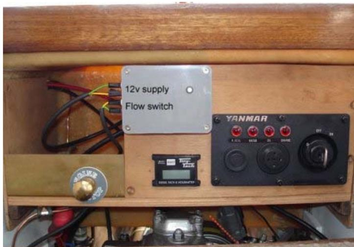
The flow switch has to be installed so that the switch unit is uppermost. The inlet hose is 1/2" inside diameter, approximately the same as the inlet on the water pump. The water inlet strainer, filter and hose I'd already fitted were 3/4" so I used a reducer on the inlet side of the flow switch.
